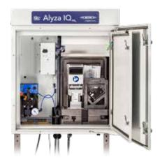
Alyza IQ PO<sub>4</sub> one channel version with open measuring unit and visible photometer
